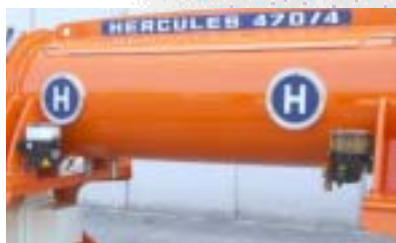
Electronic control boxes for centralised lubrication of bowl bearings and sludge scraper.
