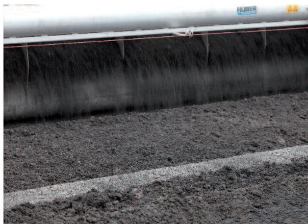
*Backmixing and aeration of sludge*
